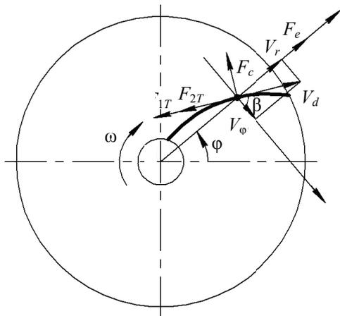
Fig. 1. Calculation scheme of particle motion over curved blades
