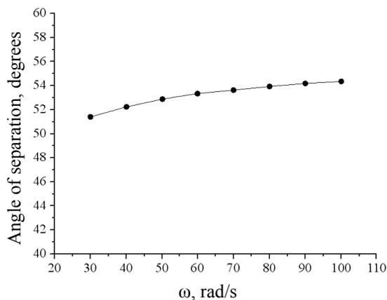
Fig. 3. The dependence of the angle of the particle separation on the angular velocity of the rotor
