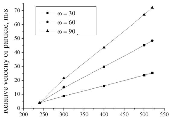
Fig. 4. The dependence of the relative velocity particles on the current radius of the rotor  $r$
