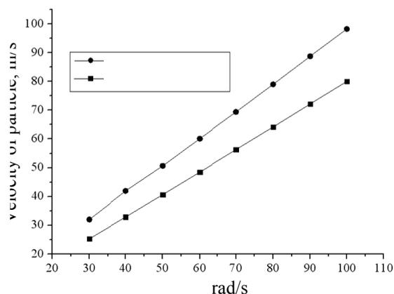
Fig. 2. The dependence of the speed of particle emission on the angular speed of the rotor
