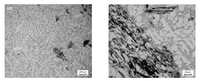
Fig. 13. The microstructure of the composite sample obtained with the use of fullerene niello after etching.
