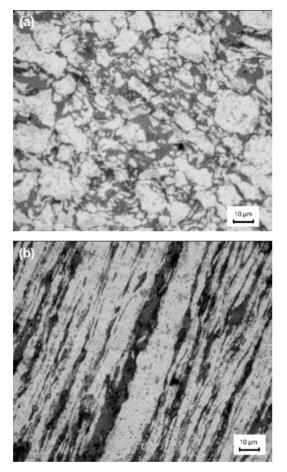
Fig. 8. The microstructure of the ligature sample Al + 10 % microcrystalline carbon: a) cross section; b) longitudinal section.
