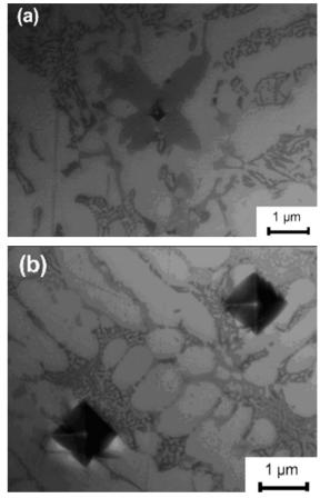
Fig. 15. Microstructure of the alloy specimen obtained using ultrafine raw materials, with imprints of the indenter: a) Hm = 8310 MPa; b) Hm = 1080 MPa, Hm = 1200 MPa.
