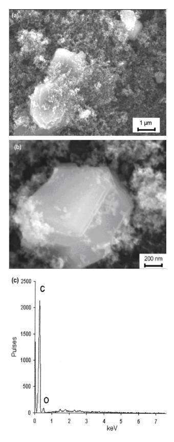
Fig. 2. Fine structure (a, b) and diagram of fullerene soot (c).
