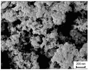
Fig. 3. Fine structure and results of EDX analysis of the powder of fullerene niello: (a) image of the area of EDX analysis; b) graph of Counts-keV; c) image of the particles in SEM.
