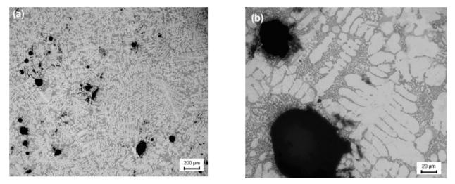
Fig. 10. The microstructure of the composite sample obtained with the use of microcrystalline carbon after etching.
