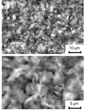
Fig. 4. Topographic images of microcrystalline powder of carbon.
