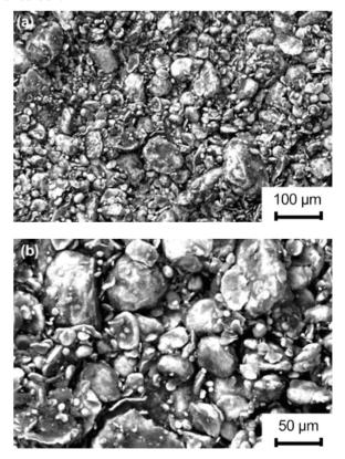
Fig. 5. Topographic images of powder charge Al + 10 % fullerene soot.
