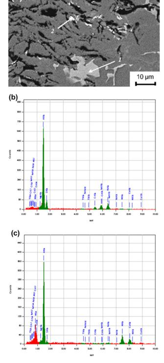
Fig. 14 – Fine structure and results of micro-x-ray spectral analysis EDX of the composite sample obtained using fullerene niello: a) image of the area of EDX analysis; b) results of micro-X-ray spectral analysis EDX at zone 1; c) results of micro-x-ray spectral analysis EDX at zone 2.
