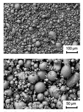
Fig. 1. Topographic images of the original aluminum powder.
