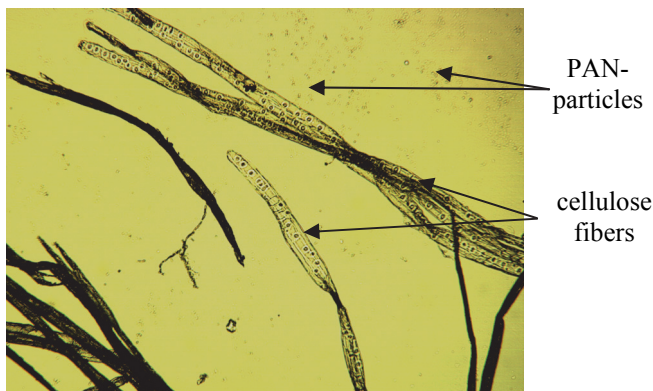
Fig. 7. Cellulose fibers and PAN-particles
