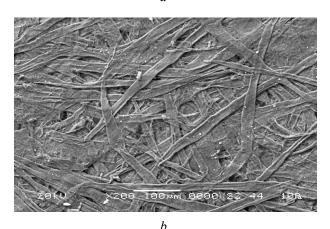
Scans the surface of the paper based on thermomechanical pulp from aspen wood: a – initial TMP; b – chemically modified TMP
