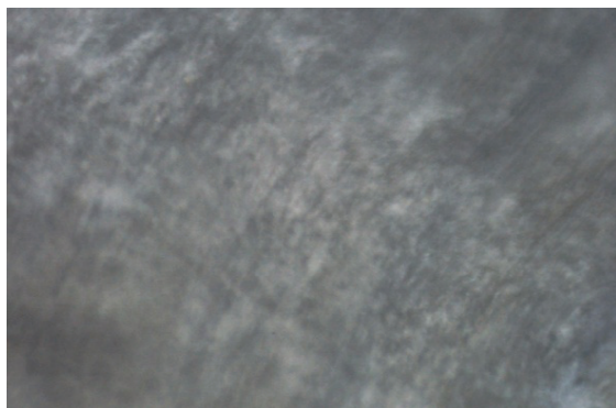
Fig. 3. An image of the surface of PE, containing 10 wt % filler VC PE 175 (magnification – 250 times)
