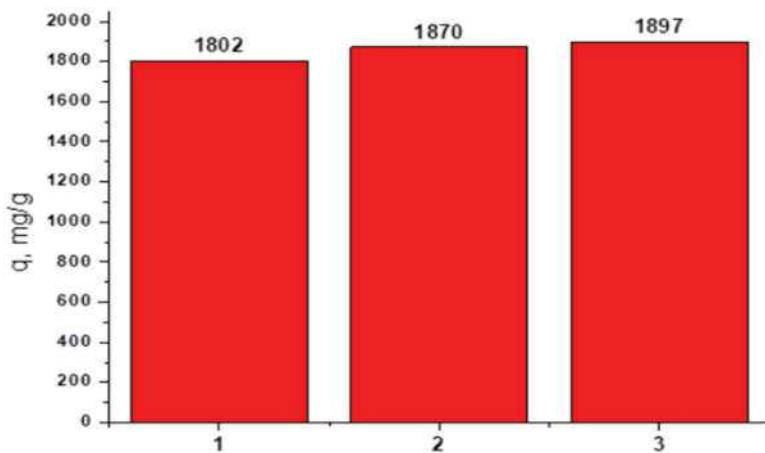
Figure – Adsorption capacity of composites toward to methylene blue: 1 – MS0.5, 2 – MS1 and 3 – MS7.
