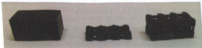
Fig. 1. Carbon filler ( a ), three-dimensional structures printed by FDM technology ( b )
