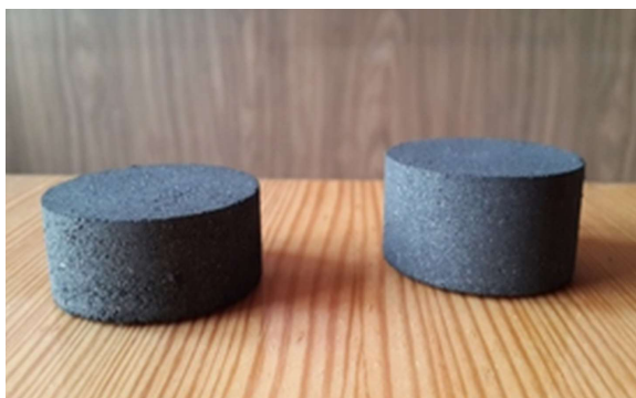
Fig. 3 Coal and coke dust briquettes with a standard urea binder.
