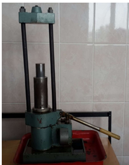
Fig. 2 The compression mold and the stamp press.
