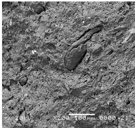
Fig.4. Electron microscopic image of the surface of the sample of ceramic tiles
