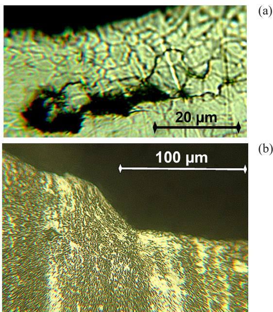
Fig. 4. Defects in the structure of the surface layer formed during the contact wear of the working surface of the samples modified by laser processing (a), and further subjected to high temperature tempering (b).
