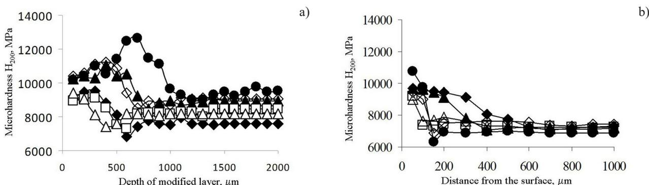
Fig. 1. Distribution of microhardness through the cross section of R6M5 steel samples for sets processed with the speed, mm/min: ● - 600, ◇ - 750, ▲ - 900, ◆ - 1050, □ - 1200, △ - 1350: a) after laser modification; b) laser modification + tempering at 560°C.
