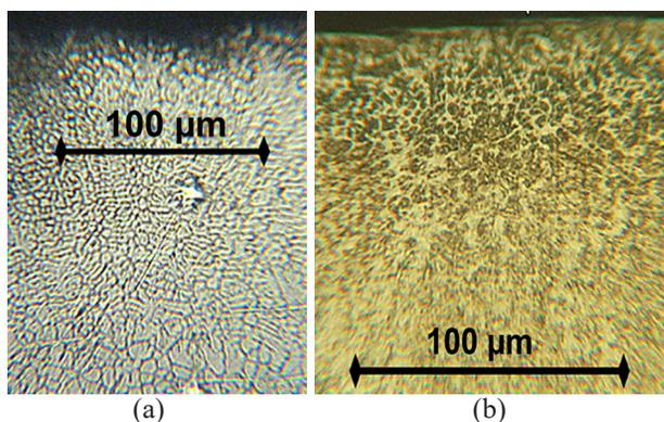
Fig. 2. Structure of the surface layer of R6M5 steel samples subjected to laser processing at a speed of 600 mm/min as a final operation (a) and after additional tempering at the temperature 560°C (b).
