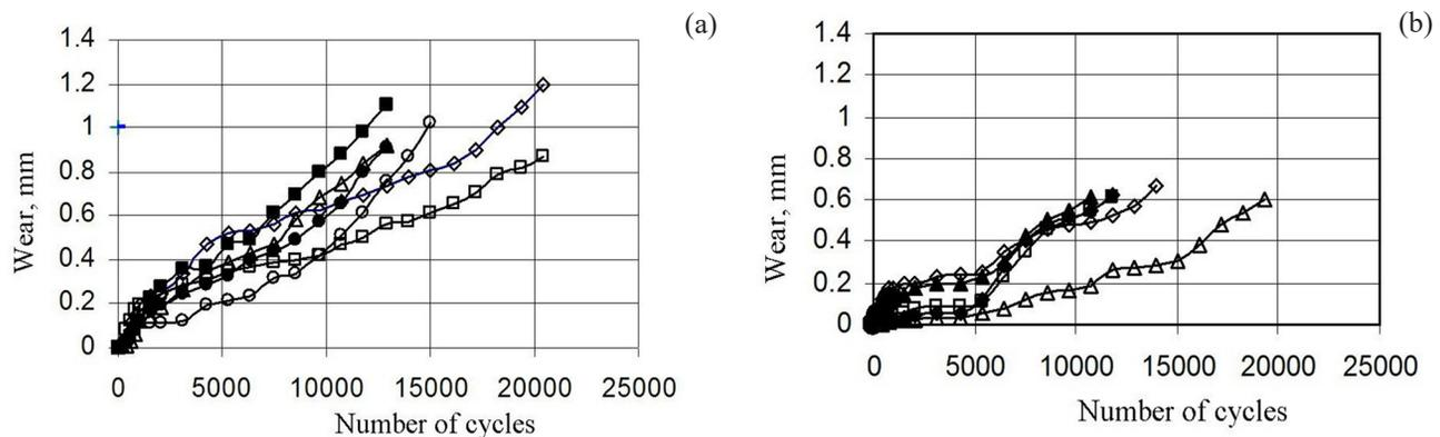
Fig. 5. Curves of the surface layer wear of R6M5 steel samples modified by laser processing (a) and after additional treatment with high temperature tempering (b).
