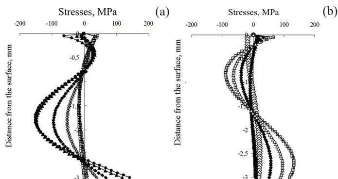
Fig. 3. Distribution of residual stresses in the modified by laser treatment of surface layer of R6M5 steel at velocities: ● - 600, ◇ - 750, ▲ - 900, ◆ - 1050, □ - 1200, Δ - 1350: a) laser modification; b) laser modification + tempering at 560°C.
