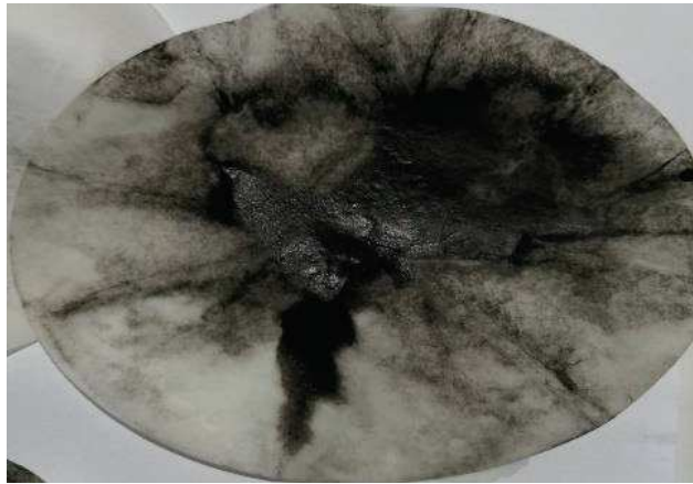
Fig. 2 - Filter with the resulting graphite particles
