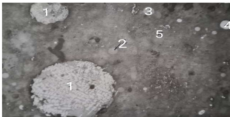
Fig.-5: Ash of Ekibastuz Coals. The light reflected, increasing 210\times 1-balls with Crystallization of Magnesite; 2- Colorless Glass Balls; 3-Yellowish-Brown Color; 4 - Black Opaque; 5-Polystyrene.
