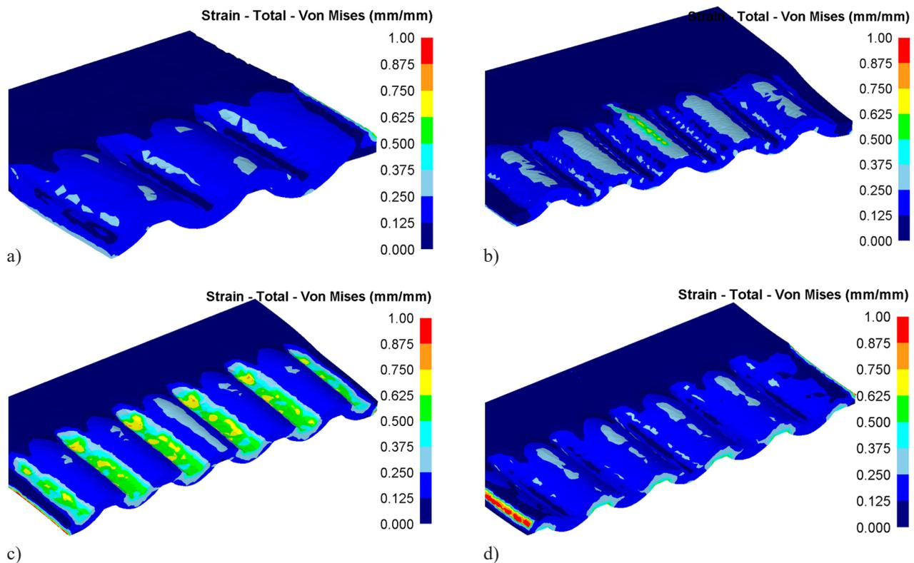
Fig. 4. Mises strain: a) - contact asymmetry; b) - geometric asymmetry; c) - kinematic asymmetry (lower face); d) - kinematic asymmetry (upper face).
