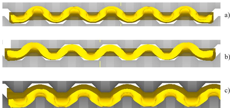
Fig. 1. Shape change in the transverse direction: a) - contact asymmetry; b) - geometric asymmetry; c) - kinematic asymmetry.
