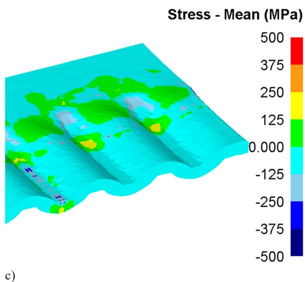
Fig. 5. Equivalent stress: a) - contact asymmetry; b) - geometric asymmetry; c) - kinematic asymmetry.
