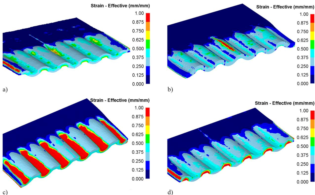
Fig. 3. Equivalent strain: a) - contact asymmetry; b) - geometric asymmetry; c) - kinematic asymmetry (lower face); d) - kinematic asymmetry (upper face).
