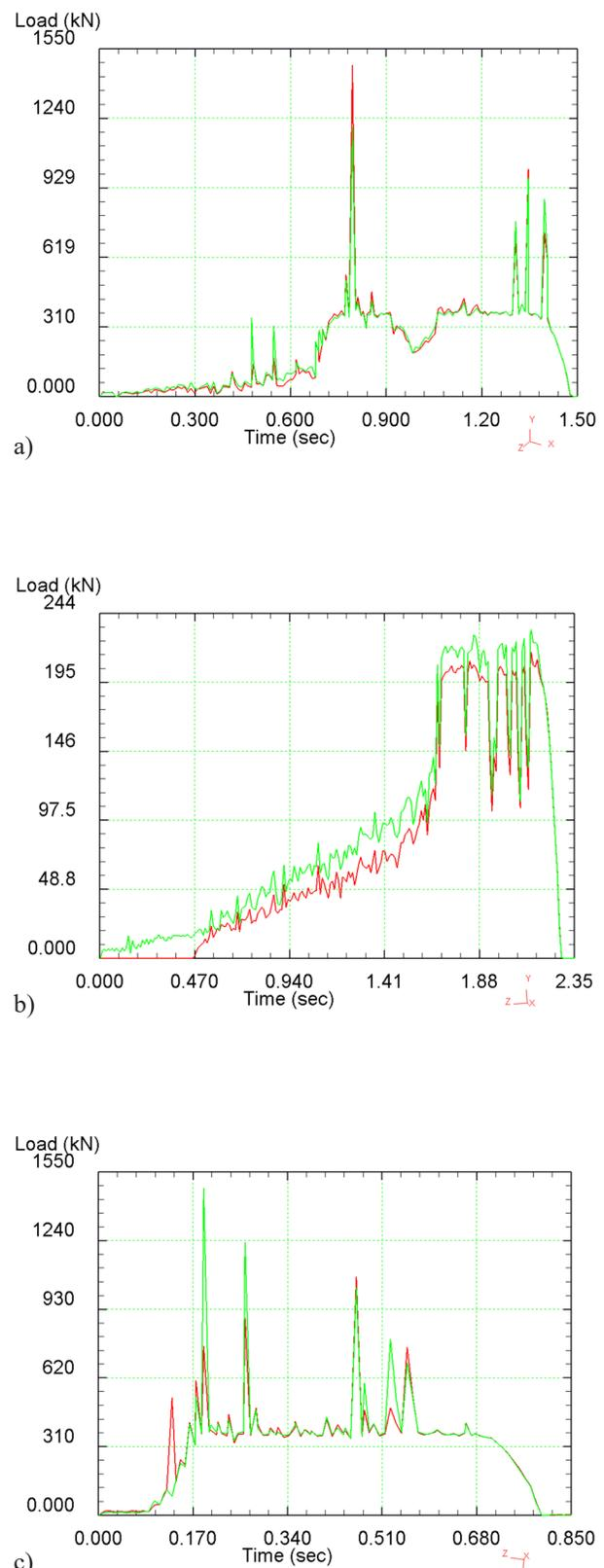
Fig. 7. Deformation force: a) - contact asymmetry; b) - geometric asymmetry; c) - kinematic asymmetry.
