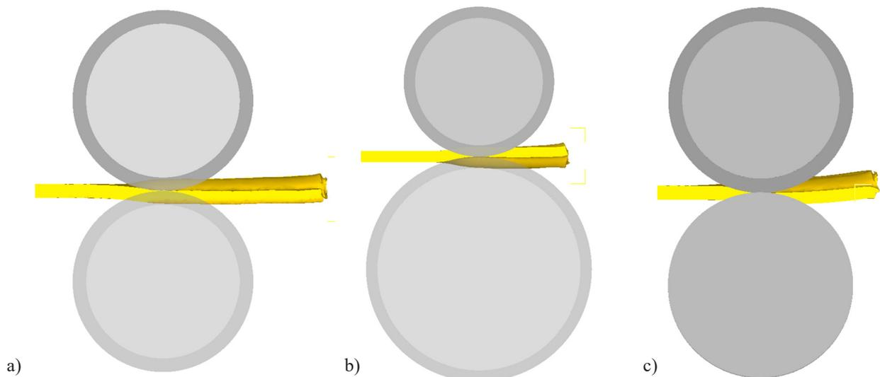
Fig. 2. Shape change in the longitudinal direction: a) - contact asymmetry; b) - geometric asymmetry; c) - kinematic asymmetry.
