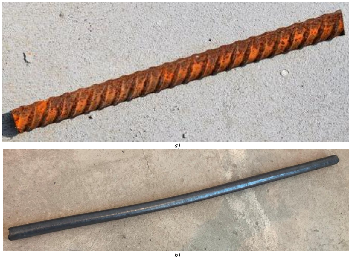
Fig. 6 Bar scrap (reinforcement profile) before (a) and after (b) rolling
