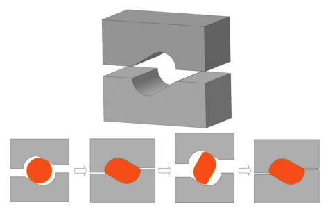
Fig. 1. Tool construction and broaching scheme in a new design forging tool.
