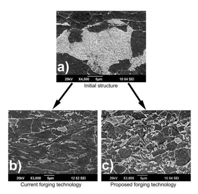
Fig. 2. Microstructure of DIN 1.2542 steel.
