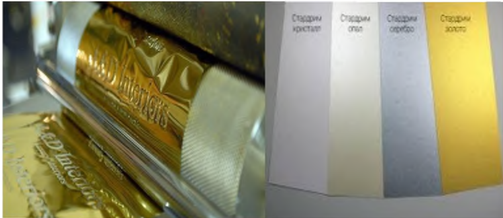
Fig 3. Hot stamping with aluminium foil and printing with metallised ink
