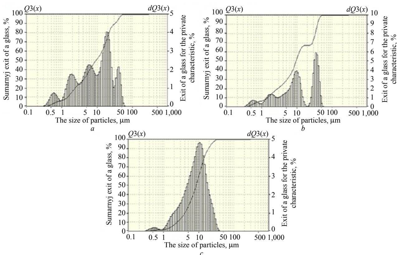
Fig. 2. The fineness characteristic of distribution of the particle size in the test volume after 15 min of grinding: a – chalk; b – kaolin; c – “white soot”
