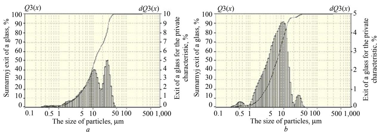
Fig. 3. The fineness characteristic of distribution of the particle size in the test volume “white soot”: a – 15 min; b – 30 min
