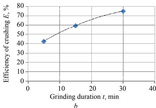
Fig. 4. The dependence of the dispersion efficiency from the impact time for the different defining sizes of particles:  $a$  – 1  $\mu\text{m}$ ;  $b$  – 10  $\mu\text{m}$
