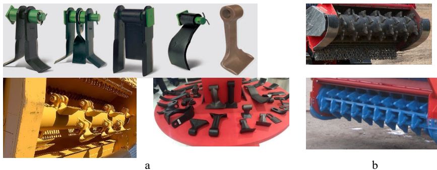
Fig. 4. Movable (a) and rigidly fixed (b) knives (hammers).
