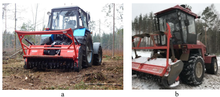
Fig. 2. Aggregation of mulchers AHWI M450m-1900 (a) and M550m-2410 (b) on the base chassis BELARUS-1221V.2 and the universal power tool UES-2-280A "PALESS 2U280A", respectively.
