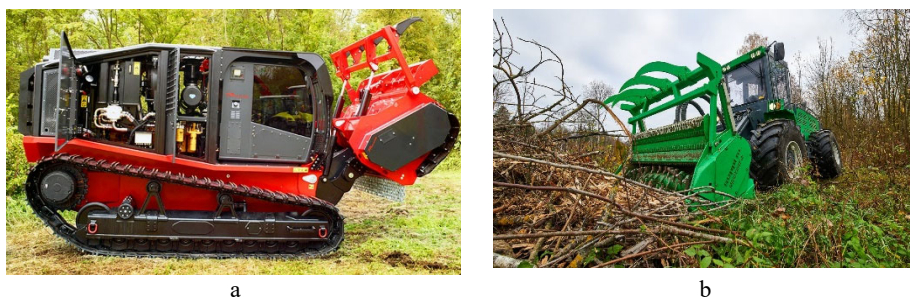
Fig. 1. Self-propelled mulchers: a - PRINOTH AHWI RAPTOR 800 (Germany), b - AMKODOR FM30A1 (Republic of Belarus).
