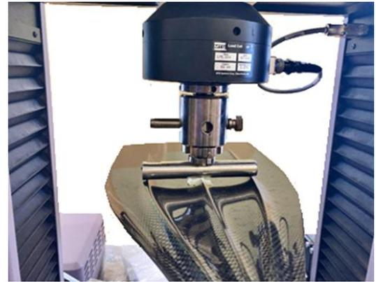
Fig. 5. Paddle blade and indenter for applying load  $F_3^a$  at point D, fixed in the grip of the MTS Criterion 43 test machine
