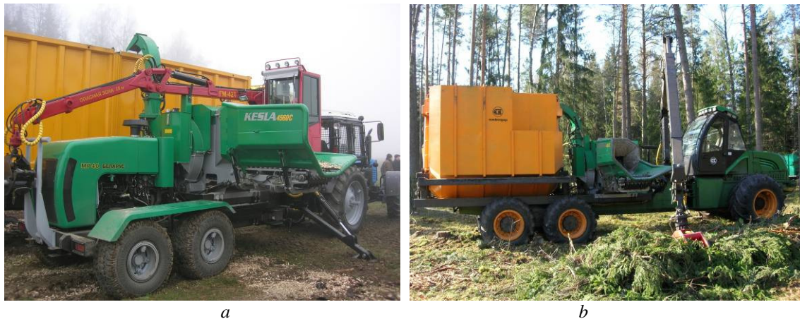
Figure 2 – Mobile barrel-type chippers with hydraulic handlers: a) driven by the stand-alone motor MR-40 (“Minsk Tractor Plant” Republican Unitary Enterprise); b) driven by the forwarder motor, with the collecting bin “Amkodor-2902” (“Amkodor” Open Joint-stock Company)
