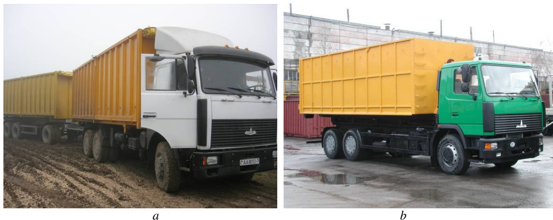
Figure 3 – Trucks for chips transportation (“Minsk Automobile Plant” Republican Unitary Enterprise): a) road train MAZ-5516+MAZ-8561; b) chip truck with “multilift” container handling mechanism MAZ-6501
