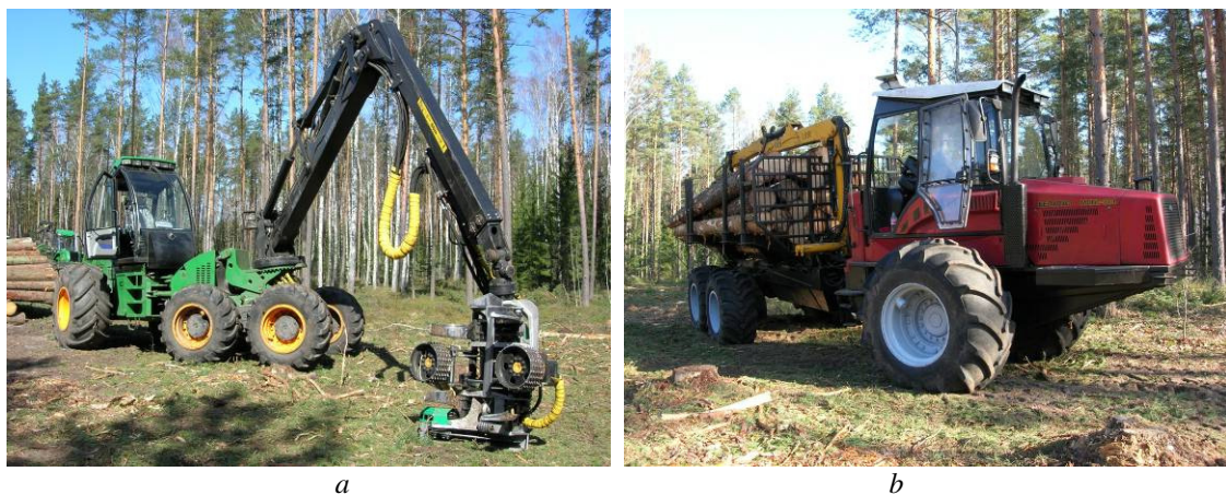
Figure 1 – Wheeled logging machines: a) harvester (“Amkodor” Open Joint-stock Company); b) forwarder (“Minsk Tractor Plant” Republican Unitary Enterprise)
